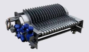
Bottle insert with one-finger-system on a crank drive. By swivelling mounting of the fingers a wear resistant one-finger-disconnection is attained.
